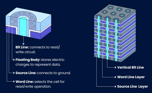
3D X-DRAM is an industry game-changer. It is based on floating body cell (FBC) technology, so data is stored as electric charges without capacitors. An innovative structure similar to 3D NAND flash makes 3D X-DRAM easier to manufacture and less expensive to scale than emerging 3D DRAM alternatives. 3D X-DRAM using multiple-level 3D arrays, so 8x higher capacities can be achieved using the same number of layers (230) used for 3D NAND.
